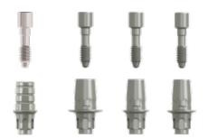
CAD-CAM blanks allow occlusally-screwed crowns and/ or individual abutments to be manufactured in the digital milling process with a precise connection structure. Adhesive abutments were developed specifically for the manufacture of individual hybrid abutments consisting of a prefabricated Ti adhesive base and an individually manufactured zirconium or pressed ceramic base using suitable 2K adhesive and are ideally suited for high-quality front tooth restoration.
